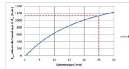
**E700 was reached with 15 kg/m<sup>3</sup> MiniBars™, and E1000 with 25 kg/m<sup>3</sup> MiniBars™, corresponding to 933 J and 1333 J according to EN 14488-5.**
