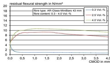
Figure 8: residual flexural strength to CMOD, mean values of: C25/30 – 0.3 Vol.-% – 43 mm, C25/30 – 2.5 Vol.-% – 43 mm and C25/30 – 4.0 Vol.-% – 43 mm
